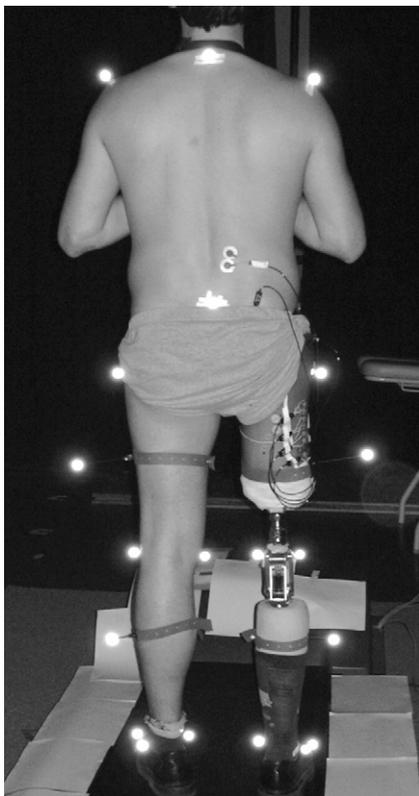
**Fig. 1.** Photograph of one of the expert amputees during standing acquisition on the treadmill. The picture also shows the specific shaft that had been developed with the purpose to acquire EMG of stump muscles using integrated electrodes.
